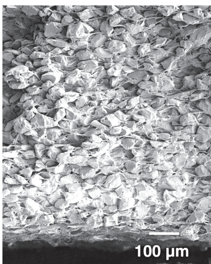
Cross section of a standard density (SD) Empore™ disk (30-60 μm particle size)
