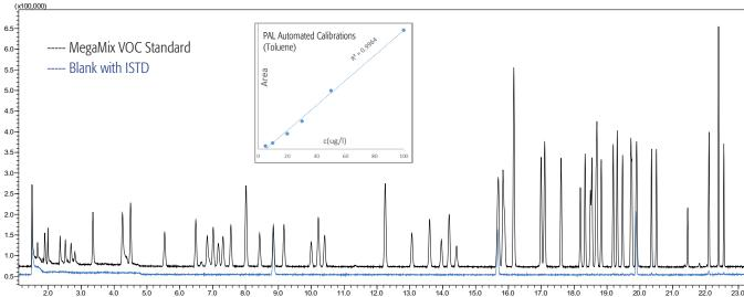
Figure 1: Chromatogram of volatiles at 20 ppb.
