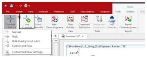
To co-add the Spectra, choose Peak(background subt) from the Crosshair Select Tool, under the CDS Ribbon. The Peak (background subt.) tool allows a user to select mass spectra of peaks to display, in which the tails of each peak are not included in the mass spectrum, to provide cleaner data.
