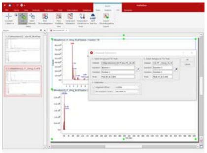
An alignment offset and a normalization factor will be automatically calculated, but can be adjusted by the user for fine-tuning. Click OK to perform the subtraction.
