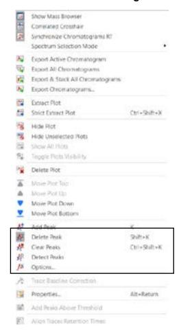
For example, to remove an integration, select "Delete Peak", Then right-click and drag over the desired area. Once the peak integration is deleted, the retention time label and the integration line will disappear:
