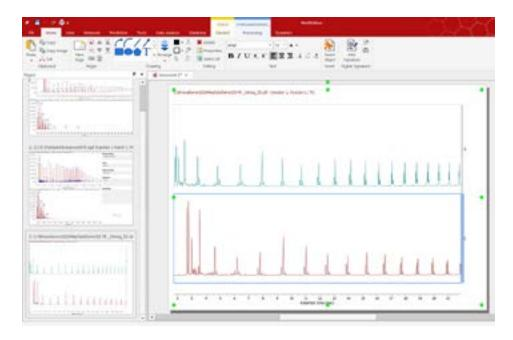
Chromatograms can be normalized by selecting the Stacked ribbon, and clicking on the Autonormalization icon.
