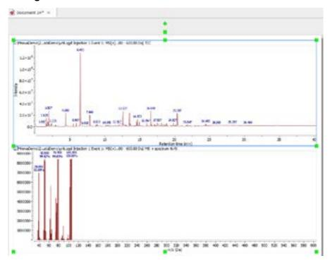
All Py-GC-MS data entries were pyrolyzed at 700°C for 30 seconds. The GC column was a 30 meter 5% phenyl with a 0.25mm l.D. and a  $0.25\mu m$  film thickness.
