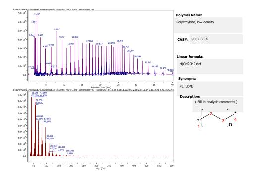
Chromatograms from the entry and the query (unknown) can be compared on the same page. This is accomplished by first pressing and holding the shift button while selecting both pages of the document in the Pages window. Then Under the CDS Ribbon and Export Chromatograms, choose "Export & Stack All Chromatograms.
