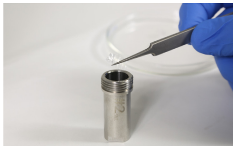
Figure 5: Cut sample to smaller pieces (<8 mm) and load into sample jar
