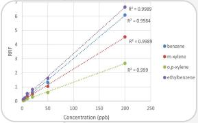
Linear calibration curves for BTEX components.
