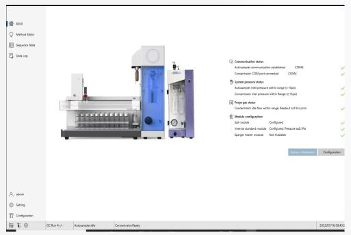
The homescreen of the 8500 uniquely provides real-time updates on system health for communications, system pressure, purge gas, and active module configuration.
