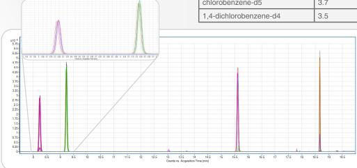
Overlay of extracted ion chromatograms for EPA 8260 internal standards at 25ppb (n=7) over 12 hours.
