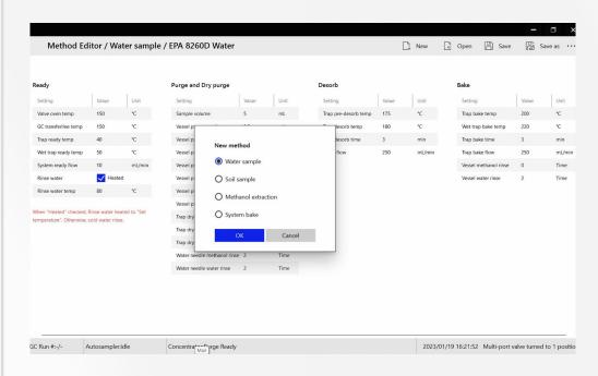
Method Editor allows users to create separate methods for not only for Water and Soil samples, but also performing Methanol Extraction and System Bake. Create your purge and trap method or use pre-loaded methods for all the critical EPA methods such as 8260, 524, and 624.
