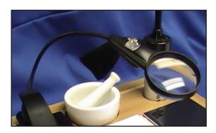
The New Sample Prep Station aids in getting your small-sized samples ready by providing a lighted magnifying glass-illuminating and enlarging your sample view on a sample prepping platform.
