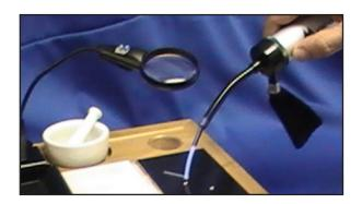
The compact vacuum pump allows you to easily draw solid samples into your quartz sampling tube.
