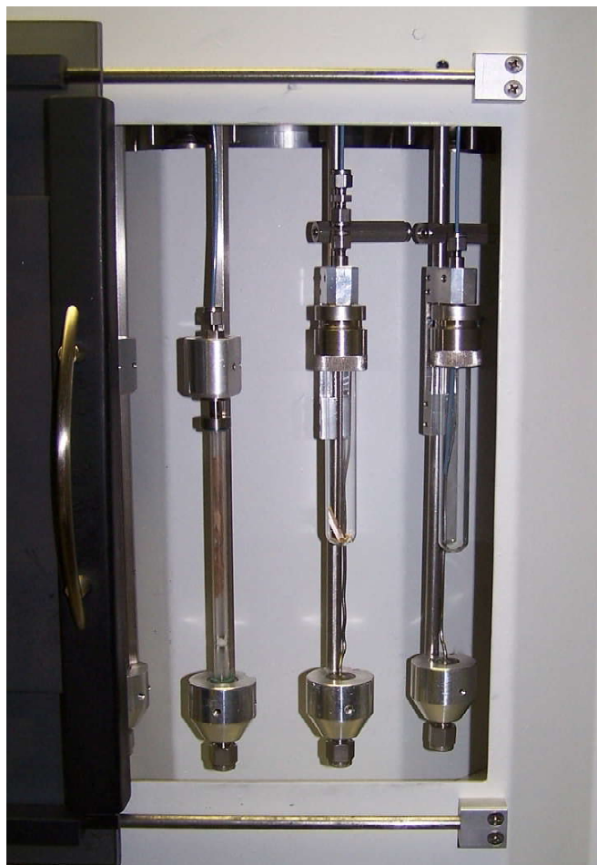
Figure 3: Thermal Desorption Autosampler with 8 mm sample tubes and Dynamic Headspace Stations
